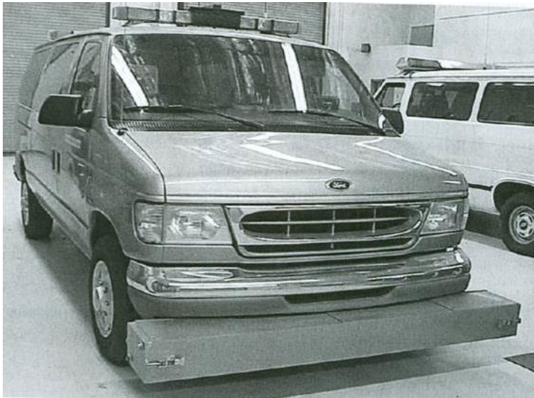
Figure 3.2. Profilometer used by the Arizona Department of Transportation to measure both ride quality and rutting
